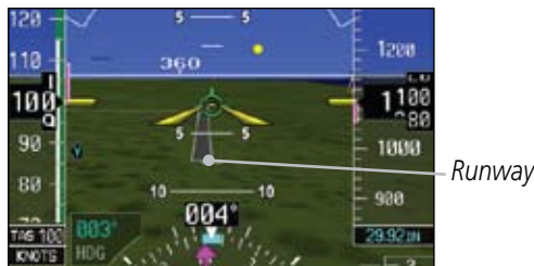
Figure 5-41 Depiction of Runway with Loaded Approach
